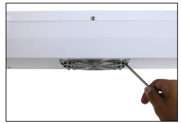
Figure 10. Shorting the ionizer's two fan grills
