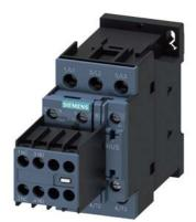
power contactor, AC-3 17 A, 7.5 kW / 400 V 2 NO + 2 NC, 220 V AC, 50 / 60 Hz, 3-pole, Size S0, screw terminal Removable auxiliary switch
