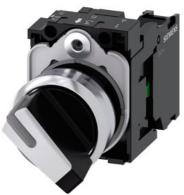
Selector switch, illuminable, 22 mm, round, metal, shiny, white, selector switch, short, 2 switch positions O-I, latching, actuating angle 90°, 10:30h/13:30h, with holder, 1 NO, screw terminal, Z=20-unit packaging
