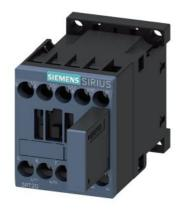
power contactor, AC-3 12 A, 5.5 kW / 400 V 1 NC, 24 V DC 0.7-1.25\* US, with varistor plugged on, 3-pole size S00, screw terminal not expandable with auxiliary switch
