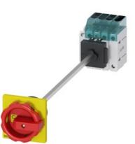
Load disconnector 3LD3, lu 16 A Main switch 3-pole + N Rated operating capacity at AC-23 A at 400V 7.5kW floor mounting Basic switch with door coupling Central hole mounting 22.5mm Rotary actuator red / yellow 66 x 66 mm with auxiliary switch 10E + 1S
