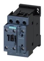
power contactor, AC-3 25 A, 11 kW / 400 V 1 NO + 1 NC, 400 V AC, 50 Hz, 400-440 V, 60 Hz, 3-pole, Size S0, screw terminal
