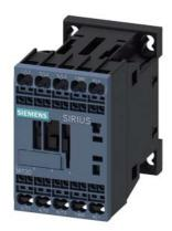
power contactor, AC-3 7 A, 3 kW / 400 V 1 NO, 24 V DC 0.7-1.25\* US, suppressor diode integrated, 3-pole, size S00, spring-type terminal not expandable with auxiliary switch
