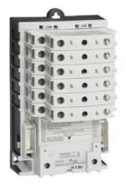
Electrically held lighting contactor, (convertible to mech. held), Amp rating 30A (tungsten 20A), 4 N.C. / 3 N.O. poles, 460-480V 60Hz/440V 50Hz coil, Non-combination type, Enclosure NEMA type (open), No enclosure
