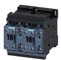
Reversing contactor assembly, AC-3, 4 kW 400 V, 24 V DC 3-pole, Size S0 screw terminal electrical and mechanical interlock 2 NO integrated
