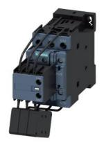
Capacitor contactor, AC-6b 25 kVAr, / 400 V 1 NO + 2 NC, 50-60 Hz AC 200-280 V DC 3-pole, Size S0 screw terminal
