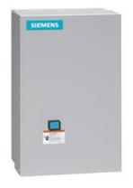
Non-reversing motor starter Size 2 1/2 Three phase full voltage Amb compensate bimetal OLrelay Contactor amp rating 60Amp Non-combination type Enclosure NEMA type 1 Indoor general purpose use Extra-wide enclosure
