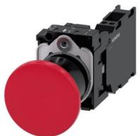
Mushroom pushbutton, 22 mm, round, plastic, red, 40mm, latching, pull-tounlatch mechanism, with holder, 1 NO+1 NC, spring-type terminal, with laser labeling, inscription or symbol Customer-specific selection with SIRIUS ACT configurator (CIN)
