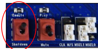
Figure 8. Left toggle switch set to “enable” position.
