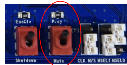
Figure 13. Right toggle switch set to “play” position.
