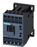
power contactor, AC-3 9 A, 4 kW / 400 V 1 NC, 24 V DC 0.7-1.25\*Us 3-pole, size S00 spring-type terminal with integrated diode, suitable for PLC outputs not expandable with auxiliary switch
