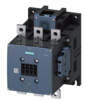
Contactor, AC-1, 400 A/690 V/40  $^\circ$ C, S10, 3-pole, 200-277 V AC/DC, PLC-IN optional, with varistor, 2 NO+2 NC, Connection rail/ screw terminal
