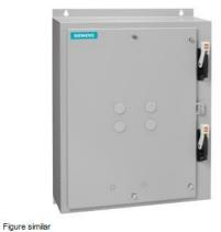
Duplex starter w/ alternator, Size 0, Three phase full voltage, Amb. compensate bimetal OLR, Contactor amp rating 18A, 110V 50Hz / 120V 60Hz coil, Combination type, Two 30A disconnect switches, Enc NEMA type 4 painted steel, Water/dust tight for outdoors
