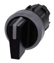
Illuminable selector switch, 22 mm, round, plastic with metal front ring, black, Selector switch short, 3 switch positions I>O<II, momentary contact type, actuating angle  $2x45^{\circ}$ , 10:30h/12h/13:30h
