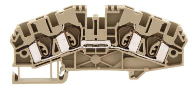
Feed-through terminal, Tension-spring connection, Mounting type: Mounting rail TS 35/7.5, Rated cross-section: 4 mm<sup>2</sup>, Width: 6.1 mm, Colour: Beige
