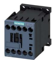
Power contactor, AC-3 12 A, 5.5 kW / 400 V 2 NO + 2 NC 48 V DC 4-pole Size S00 screw terminals
