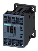
power contactor, AC-3 7 A, 3 kW / 400 V 1 NO, 24 V DC 0.85-1.85\* US, with diode integrated, 3-pole, size S00, spring-type terminal not expandable with auxiliary switch
