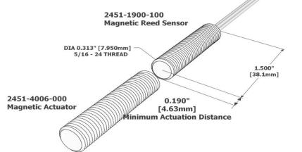
All measurements are in Inches [millimeters]
