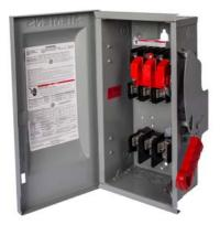
Siemens Low Voltage Circuit Protection Heavy Duty Safety Switches. Type: ENCLOSED, SAFETY SWITCH Std: UL V. Rating: 600VDC A. Rating: 60A Wattage: 3W No. Of Poles: 3P F. Rating: 60Hz Action: SINGLE THROW Material: 304SS Enclosure: TYPE 3R. 2-3 point mounting holes. O. Cycles: 10000 O. Temperature: (-20F-120F) AMBIENT TEMPERATURE Environmental Conditions: OUTDOOR
