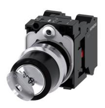
RONIS key-operated switches, 22 mm, round, metal, shiny, lock number SB30, with 2 keys, 2 switch positions O-I, latching, 90° operating angle, 10:30/1:30 o'clock, key removal O, with holder, 1NC, 1NC, spring-type terminals, possible special locks: SB31, 421, 455, Z=20-unit packaging
