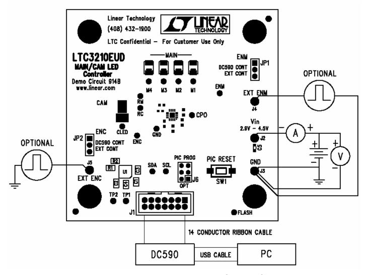
Figure 1. Proper Measurement Equipment Setup for DC914
