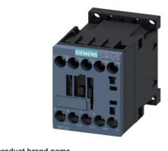
power contactor, AC-3 7 A, 3 kW / 400 V 1 NC, 24 V DC 0.85- $1.85^{*}$  US, 3-pole, size S00, screw terminal not expandable with auxiliary switch
