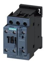
Contactor, 10 hp, 460 / 575 V, 1 NO + 1 NC, 208 V AC, 50 / 60 Hz, 3-pole, Size S0, screw terminal
