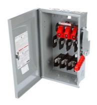
Siemens Low Voltage Circuit Protection Heavy Duty Safety Switches. Type: ENCLOSED, SAFETY SWITCH Std: CSA V. Rating: 600V A. Rating: 60A Wattage: 3W No. Of Poles: 3P F. Rating: 60Hz Action: SINGLE THROW Material: STEEL Enclosure: TYPE 1. 2-3 point mounting holes. O. Cycles: 10000 O. Temperature: (-20F-120F) AMBIENT TEMPERATURE Environmental Conditions: INDOOR
