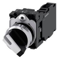
Selector switch, illuminable, 22 mm, round, metal, shiny, white, selector switch, short, 2 switch positions O-I, latching, actuating angle 90°, 10:30h/13:30h, with holder, 1 NO+1 NC, screw terminal
