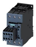
Power contactor, AC-3 80 A, 37 kW / 400 V 2 NO + 2 NC, 20-33 V AC/DC with varistor 3-pole, size S2 screw terminals
