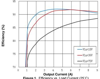
Figure 1. Efficiency vs. Load Current (25°C)
