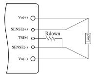
Figure 15. Circuit to Decrease Output Voltage
