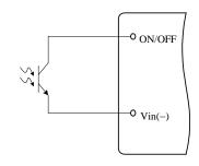
Figure 12. Opto Coupler Enable Circuit
