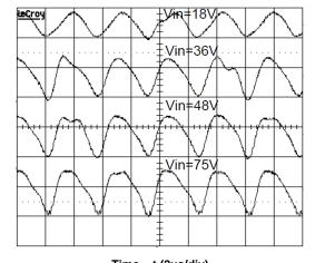
Output Voltage Ripple (50mV/div)
