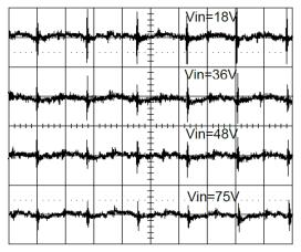
Time - t (2µs/div) Figure 6. Input Reflected Ripple Current at Full Load
