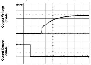
Time - t (1ms/div) Figure 3. Start-Up from Enable Control (typical Vin and full load)
