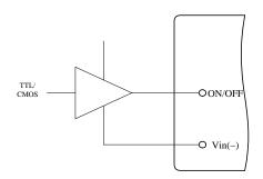
Figure 14. Direct Logic Drive
