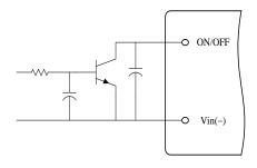
Figure 13. Open Collector Enable Circuit
