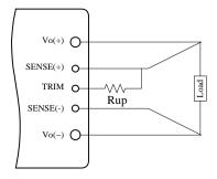
Figure 16. Circuit to Increase Output Voltage
