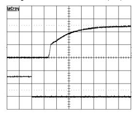
Time - t (1ms/div) Figure 4. Start-Up from Enable Control (typical Vin and zero load)
