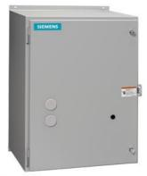
Mechanically held lighting contactor, Contactor amp rating 200A, 0 N.C. / 2 N.O. poles, 110VAC 50HZ/120VAC 60HZ coil, Non-combination type, Enclosure NEMA type 12, Dust/drip proof for indoors
