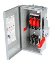
Siemens Low Voltage Circuit Protection Heavy Duty Safety Switches. Type: ENCLOSED, SAFETY SWITCH Std: UL V. Rating: 600V A. Rating: 30 A Wattage: 4W No. Of Poles: 3P F. Rating: 60Hz Action: SINGLE THROW Material: 304SS Enclosure: TYPE 3R. 2-3 point mounting holes. O. Cycles: 10000 O. Temperature: (-20F-120F) AMBIENT TEMPERATURE Environmental Conditions: OUTDOOR
