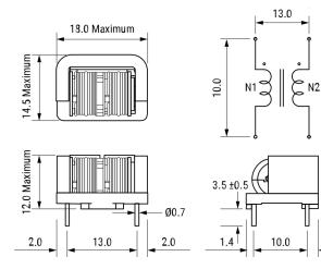
General InformationSeriesSSRH7HS-MStyleThrough-HoleRoHSYesNotesM10 Lot No.MiscellaneousTemperature Rise Maximum: 50 K.CoreMn-Zn Ferrite
