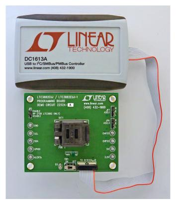
Figure 3. DC1613A Ribbon Cable Installation
