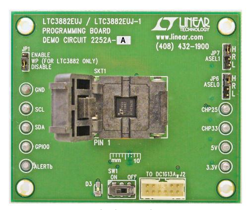
Figure 2. Open Shell. Verify IC Installed
