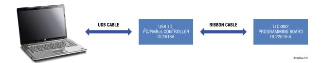
Figure 1. LTC3882 Programming Setup Using DC2252A-A
