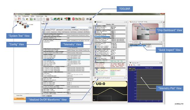
Figure 4. LTpowerPlay Interface of Programming the LTC3882
