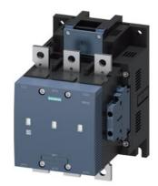
vacuum contactor, AC-3 300 A, 160 kW / 400 V, AC (50-60 Hz) / DC operation 23-26 V AC/DC auxiliary contacts 2 NO + 2 NC 3-pole, frame size S10 busbar connections drive: conventional
