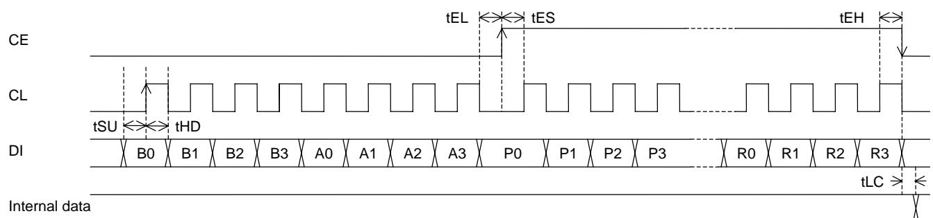
**Serial data output (OUT) tSU, tHD, tEL, tES, tEH  $\geq 0.75\mu s$  tDC, tDH <  $0.35\mu s$**
