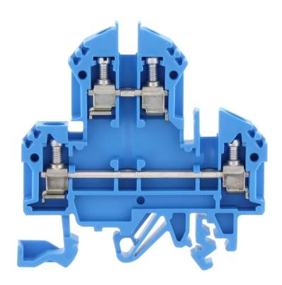
Double-level terminal, Screw connection, Mounting type:Mounting rail TS 35/7.5 and TS 32, Rated cross-section: 4 mm², Width: 6 mm, Colour: Blue
