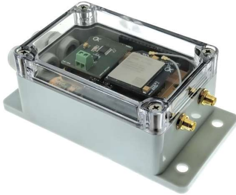
Pic. 22. LTE GPS BG96 tracker with RS485 port (LLS sensor)
