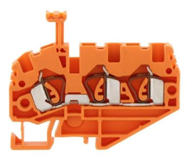
Feed-through terminal, Tension-spring connection, Mounting type: Mounting rail TS 15/5.5, Rated cross-section: 2.5 mm<sup>2</sup>, Width: 5.1 mm, Colour: Orange
