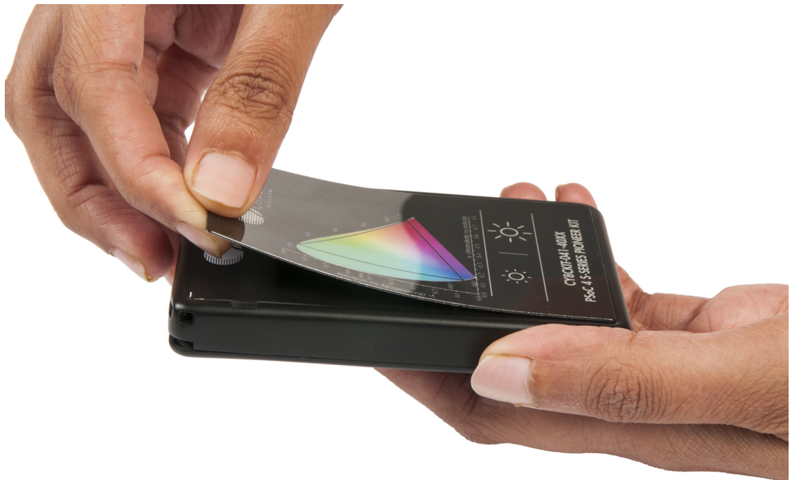
Figure 3-10. Removing the Overlay
