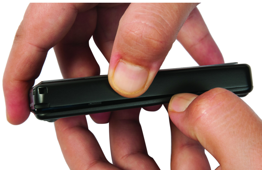
Figure 3-7. Removing the bottom case
