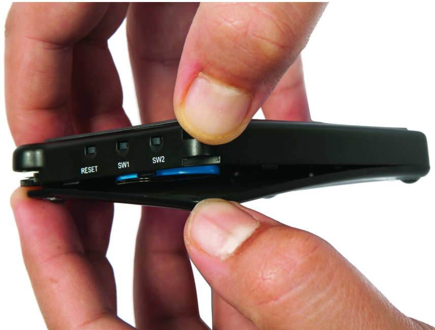
Figure 3-6. Opening the bottom case
