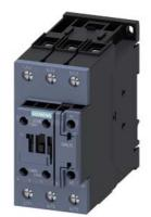
power contactor, AC-3 51 A, 22 kW / 400 V 1 NO + 1 NC, 200 V AC, 50 Hz / 200-220 V, 60 Hz 3-pole, size S2, screw terminal
