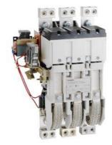
Mechanically held lighting contactor, Contactor amp rating 400A, 0 N.C. / 3 N.O. poles, 440VAC 50HZ/480VAC 60HZ coil, Non-combination type, Enclosure NEMA type (open), No enclosure
