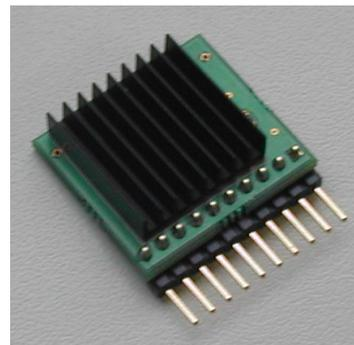
**Figure 4. Adding a Heat Sink to Improve Cooling**
