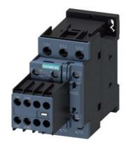
power contactor, AC-3 25 A, 11 kW / 400 V 2 NO + 2 NC, 230 V AC, 50 Hz, 3-pole, Size S0 screw terminal Removable auxiliary switch
