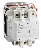
Mechanically held lighting contactor, Contactor amp rating 200A, 0 N.C. / 3 N.O. poles, 110VAC 50HZ/120VAC 60HZ coil, Non-combination type, Enclosure NEMA type (open), No enclosure
