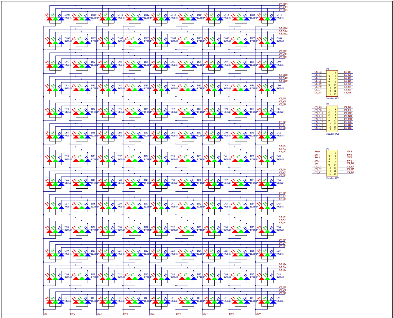
Figure 4: FxLED_9x13_ARRAY Application Schematic
