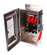
Siemens Low Voltage Circuit Protection Heavy Duty Safety Switches. Type: ENCLOSED, SAFETY SWITCH Std: UL V. Rating: 240V A. Rating: 30 A Wattage: 3W No. Of Poles: 3P F. Rating: 60Hz Action: SINGLE THROW Material: SS Enclosure: TYPE 4X. 2-3 point mounting holes. Insulation: YES O. Cycles: 10000 O. Temperature: (-20F-120F) AMBIENT TEMPERATURE Environmental Conditions: INDUSTRIAL CORROSIVE RESISTANCE
