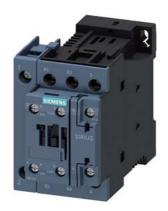
Power contactor, AC-3 25 A, 11 kW / 400 V 2 NO + 2 NC 125 V DC 4-pole size S0 screw terminals 1 NO + 1 NC integrated
