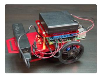
Finish the robot by screwing the top plate firmly to the standoffs in the center. Use double sided foam tape or electrical tape to hold the 4xAA battery pack to the top plate, and the USB battery pack to the front of the robot.
