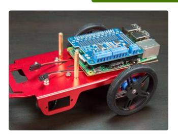
Push the motor HAT into place on the Pi's GPIO connector. Screw down the standoffs if being used to hold the HAT.
