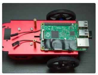
If you aren't using Pi HAT standoffs to hold the motor HAT place a piece of electrical tape across the HDMI connector side of the Pi. This will help prevent the motor HAT from getting pushed down into the connectors and shorting out. If you are using the standoffs you can place them over the front mounting holes of the Pi (not shown).
