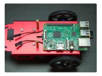
Place the Pi on the cardboard and position it so the Pi's rear mounting holes (near the USB ports) are directly above the long mounting slot at the back of the chassis. Use the #4-40 machine screws and nuts to screw through the Pi and cardboard to securely hold the Pi in place.
