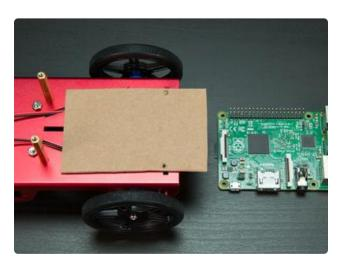
Cut out a small square of cardboard that's about the same size as the Raspberry Pi. This cardboard will protect the bottom of the Pi from touching the metal robot chassis and shorting out. It's very important to prevent the bottom of the Pi from touching the metal chassis or you could damage the Pi!
