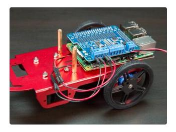
The left (or 'driver side' for US/right side of the road drivers) DC motor should be connected to port M1 on the motor HAT.
