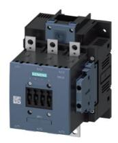
power contactor, AC-3 150 A, 75 kW / 400 V AC (50-60 Hz) / DC operation 575-600 V AC/DC auxiliary contacts 2 NO + 2 NC 3-pole, frame size S6 busbar connections drive: conventional screw terminal
